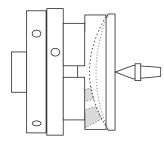
Mark the centre of the flat side of the jewellery wood (which is still square at this stage). Place the tailstock centre at this point and move the tail and wood up to the chuck.
