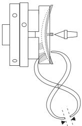
Hold the wood firmly in place. Cut it to the thinness required except for the tailstock support in the middle. Measure the wood thinness and check for even thickness before removing the tailstock. Remove the tailstock. Check that the jewellery wood remains well secured by the double-sided tape. Cut or sand away the centre piece. Sand to a fine finish.
