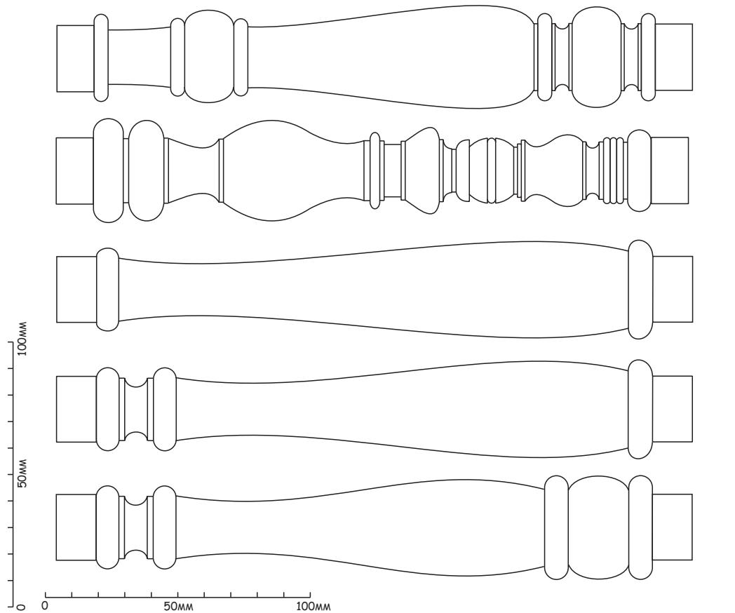
Pseudo-cabriole. Make the wood round and turn the beads. Then turn with each end off-centre while the other end is on-centre as shown below. The off-sets are on opposite sides. For a tapered cabriole cut the wood to a taper before shifting off-centre.
