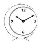
Make two pivot pins to attach the clock to the crescent. These should be a firm fit in the drilled holes. Then the holes through the crescent will need to be eased. Make a foot, with a small flat on top, for the clock to stand on.
