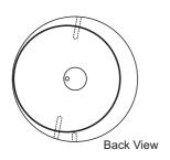
Mount the wood on a screw chuck in the off-centre hole with the face of the clock towards the headstock. Use a narrow parting tool to cut a groove square to the wood and almost through to the clock face. Take the wood off the lathe and bandsaw around this same line to separate the crescent from the clock.
