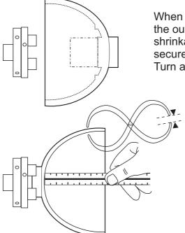
When the rough-turned blank is dry, remount it so that the outside can be turned. If there has been a lot of shrinkage this may require several re-mounts before a secure mount on the inside of the bowl is achieved. Turn and finish the outside of the bowl.
