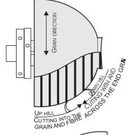
Mount the wood with the side that will become the top towards the headstock of the lathe. Use a faceplate, screw chuck or expand a scroll chuck into a drilled hole. Round the block off and make a spigot for re-mounting. This spigot should be larger than the ideal spigot size to allow for shrinkage. Shape the outside. Finishing cuts should be downhill for the best finish and you should still aim for the least end-grain tearout at this stage.
