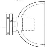
Plan the inside to have a spigot or dovetail for re-mounting when the wood is dry. The position and size of this will depend on the chuck you have to use. Allow for shrinkage when determining the size of this cut. After drying you will need to re-mount the bowl by this inside grip to finish turn the outside just as you would when turning a bowl from dry wood.
