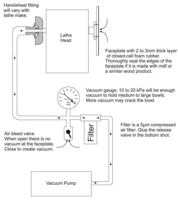
Vacuum pump should move about 9 m³/hr. A smaller pump can be improved by the addition of reserve tanks.
