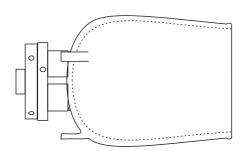
Mount the wood in a chuck, true up the face, and hollow it. Cut away the ring of wood at the leg area so that only three legs remain. Sand all surfaces. Wet sanding is recommended. When wet some woods react with steel to leave black marks on the wood. If this is likely, wrap the spigot and cover the chuck face with masking tape. Use regular sandpaper, not wet and dry, as carborundum particles can leave black marks on the wood.
