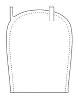
Remove the wood from the lathe. Take the spigot off using hand tools. Sand the bottom. Set the piece aside to dry. After that further finishing may be needed.
