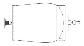
Cut the outside shape with the widest point at about one third up the bin. Leave a ring of wood around the bottom that can be cut back later to leave three legs. Turn a spigot for a 130mm deep jawed chuck. Plan the curve of the bottom so that the legs will be at least 10mm below the curve of the bottom. To check continuity of curve between the side and bottom it can be easier to carve away a little of the ring of wood that will be the feet.
