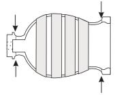
Take the wood out of the chuck and carefully saw off the foot and the waste rim as shown by the arrow in the drawing to the left. Remove the binding tape. The three pod carpels should fall free from the waste wood.
