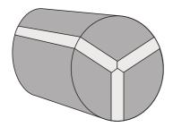
Apply glue to the faces to be joined but put no glue on the area that is to be the finished pod - the white part in the drawing above. It is very important that these faces of the finished pod do not stick to the waste wood.
