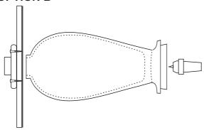
Hold the work against a rubberised faceplate using the tailstock. Cut most of the wood away using a chisel. Hand finish the remaining central area.
