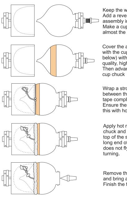
Keep the work mounted in a chuck. Add a reverse adaptor and mount this assembly in the tailstock. Make a cup chuck which will fit to almost the largest diameter of the work.
