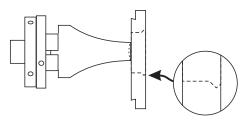
Re-mount the plastic the other way around but this time using the offset drilled hole. Cut a shallow but sharply-angled dovetail into this face. The widest point within this dovetail should be 41mm and this point should be less than 2mm back from the face of the plastic. Part the plastic off by driving a parting tool through behind the dovetail to make a 39mm dia hole.
