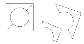
Cut through the template material. This cut must be exactly up to the inside of the line you drew and exactly at right angles to the face of the template material. With this circle of template material cut away from the central part you can now saw it to a hemisphere by cutting exactly on one side of a diagonal line. Or cut it to any other part of a circle that you need.
