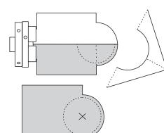
Remount in a chuck and cut the emerging part to an exact hemisphere. Use a template to ensure a perfect hemisphere and the correct dimensions. Sand this surface.
