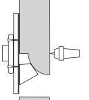
Attach the wood to a faceplate. Hot melt glue is recommended. To ensure that the centre of the box is at the centre of the faceplate bring the tailstock up to the central mark you made. Add glued-in support blocks around the emerging box.
