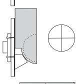
Hollow the bottom of the box. Make yourself a template to ensure an exact internal hemisphere and correct wall thickness. If you want a lip within the rim to fit the lid, cut it now. Sand and finish the inside.
