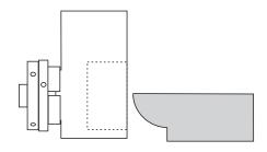
Remount on a chuck. Cut a hole on the face side to the exact diameter of the outside of the box bottom. Internally this can be square (as shown side-view here) and deeper than half the diameter of the box bottom.
