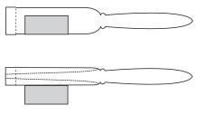
Glue a small block to one side of the blade so that the blade stands perpendicular to the workbench. Draw on the upper surface where you intend to make bandsaw cuts to create the blade.
