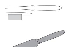
Finally, cut the side closest to the gluedon block. Sand both sides of the blade.
