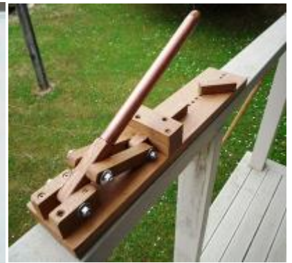
Pen press designed and made by Bruce (plans at www.sawg.org.nz )
