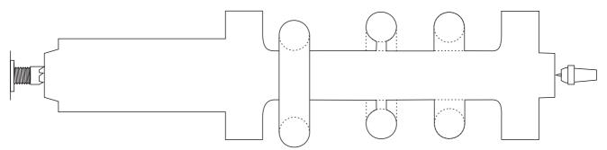
Shape the remaining areas of the rattle. Round off all corners and thin down the head and tail supports. Sand the entire surface. If a finish is used be sure that it is perfectly food-safe.
