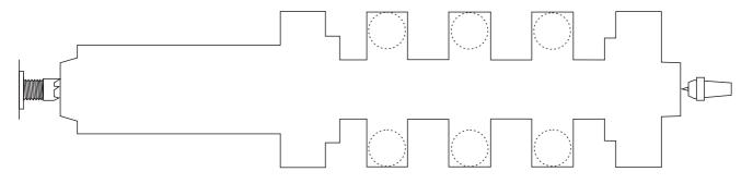
Make the three captive rings and complete the shaft in that area.
