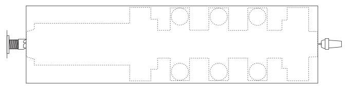
Mark the locations of the various features. Cut these down to the required diameters.
