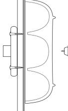
Re-mount on a vacuum chuck, Cole jaws, or pressed to a faceplate. Clean off the bottom. Sand and finish.
