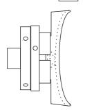
Cut the diameter of the top down to the exact size required to fit the bottom.
