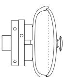
Jam fit the lid. Finish the top side of the lid. Take the lid off and ease the rim of the bottom so that the lid is no longer a tight fit.
