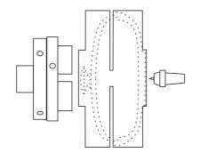
Mount the chosen wood between centres. Round it off and make a chuck bite spigot on both sides.
