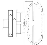
If the spigot on the underside of the box is to be retained as the foot then you may completely finish the part that is to be the underside of the box before parting it off. Part the two halves of the box. Set the bottom part of the box aside.
