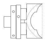
Mount the lid part in a chuck and completely cut and finish the inside.
