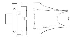
Remount the base part in a chuck. Cut the outside so that it is a jam chuck for the lid.
