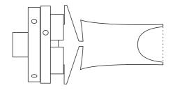
Hollow and finish the inside of the bottom part to be just a small cavity.
