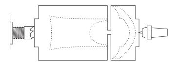
Mount your chosen wood between centres. Round it off. Cut a spigot on both ends. Part it off to separate the lid and base you will make. Set The base part aside.
