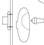
Mount a large faceplate of mdf on the lathe and glue the work piece to this.
