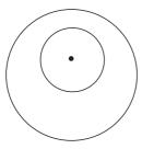
Take the wood off the lathe and work out exactly where the centre of the offset bowl is to be. Mark this point clearly.
