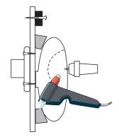
Add hot melt glue around the foot of the bowl. Add wedges and hot melt glue them to the mdf faceplate and the bowl. Later you will have to remove the support of the tailstock so be sure that the hot melt glue will hold the bowl to the mdf faceplate.
