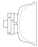
Remount in a scroll chuck. Hollow the bowl. Ensure that the lid fits loosely into the bowl.
