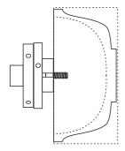
The bowl may be mounted on a drilled dovetail, small faceplate, or, as shown, a screw chuck.
