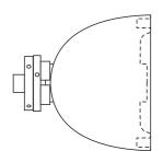
With the bowl mounted in a chuck cut a trench for the resin. Be sure that this is wide enough for the planned inserts. This trench needs to be a square cut, or a little wider at the bottom to ensure that the resin stays in place. Make the sides and bottom of the trench a nice smooth finish.
