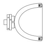
Turn the bowl over, hollow the inside, and cut the bowl rim to shape. Sand and finish the inside. Sand the resin further to 2000 grit. Then polish the resin with 3M Perfect-It 3000 Extra Cut Rubbing Compound, or one of the many other polishing compounds available.
