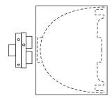
Start by creating a spigot (or dovetail) on both sides of the wood. The foot of the bowl needs to be flat or concave to ensure that the bowl will sit level on a table while the resin is setting. Then rough turn the outside of the bowl. You may finish the outside but commonly some resin will get onto that surface and require re-finishing later in the process.
