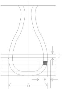
Next the angle of the sector and the minimum radial length has to be worked out to enable cutting of each segment to proceed. To do this draw each layer with a plan view as below, using the diameter A.
