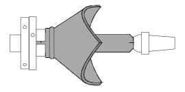
Hollow out as for a normal bowl, leaving the base a little bit thicker than the walls to provide a bit more stability when your masterpiece is on display. Sand through all the grades, the points have to be done by hand, whilst power sanding can be done below the gap areas. Finish off with your favourite polish.
