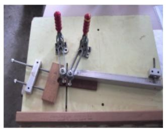
When all the segments for one layer are cut they are checked for fit and appearance using a tensioned strap to pull them into a circular shape. (See diagram below). If all is OK, the segments can now be glued together with aliphatic PVA, firstly in pairs, then glue two pairs and so on until you have 2 halves. Leave these halves overnight to set firmly before sanding the two ends of the halves square to get a good fit when glued to form the final circle.
