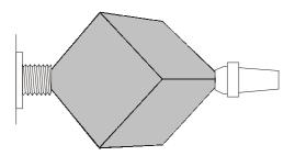
end. Should the wood slip, then re-tighten the tailstock further. Form a spigot as in the drawings; measurements will depend upon the details of your own lathe. For the Nova scroll chuck, a gripping point measurement of 43 mm for hardwood, or up to 45 mm for less dense wood will provide a perfect grip without leaving jaw marks, though usually I cut off the spigot when the turning is all complete.
