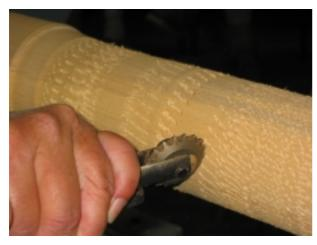
Next she added liming wax while noting the shoe polish and other coloured additives that fill the pattern made by the texturing tool are also good.
