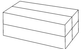
Dress four lengths of wood so that they have a square cross section. Glue them together with paper joints.
