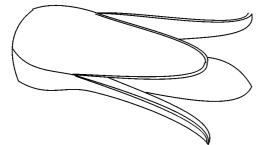
Put this glued block back on the lathe and turn the outside of the flower petals. Sand and finish.
