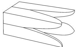
Break the paper joints apart and reglue the blocks with permanent glue in the form shown
