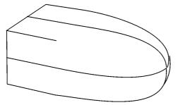
Mount this block on the lathe so that you can turn it to the shape shown. Sand and finish the surfaces that have been turned.
