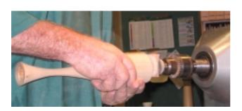
Remove the tailstock and cut a gentle curve into the top end. For the candle holding cup drill a 24mm diameter hole down to 25mm below the surface of that curve. Cut a small rebate to take the lip of the cup. Sand the top surface.
