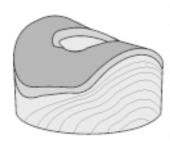
Cut a flat into the surface that is to be the upper side of the bowl. Take care not to damage the bark that will be the bowl edge. This flat can take a faceplate, screw chuck or chuck dovetail.
