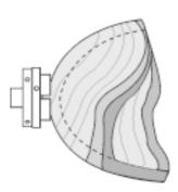
Turn the wood over and hollow it out just as you would a normal bowl. If a thin wall is planned then cut to that thickness step by step to ensure there is support for the area being cut.
