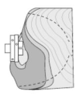
Mount the block on the faceplate, screw chuck or chuck and cut the outside shape. This wood will be out of balance so take care with lathe speed. At the bark edge it may be necessary to cut uphill a little so that the cutting action presses the bark towards the wood rather than away from the wood.
