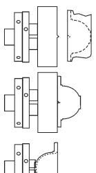
Sand flat the broad face of a deer antler button. which is to be the bottom of the box. Drill a small dent at the centre point.
