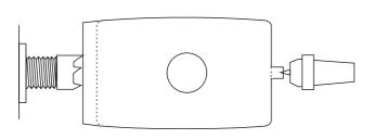
Finish the outer end down to a small central spigot.
