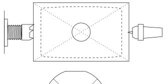
Mount this block between centres. You do not need to round it of completely. Turning the offsets later will take away about one quarter of the width, ie one eighth either side of the centre line of the original flat face.
