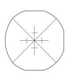
Remount the block between centres with both head and tailstock at the offset markers to the same side of centre. Turn that face just up to the longitudinal pencil marks. Repeat for each face. Sand the faces longitudinally to preserve the line between the faces.
