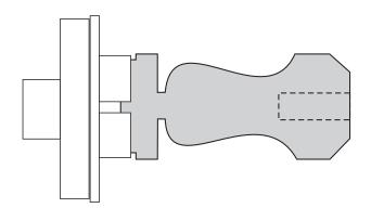
Work on towards the headstock creating the shape of your choice. When the headstock end is narrowed ready for final parting off, sand and finish the work.
