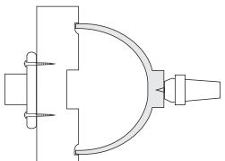
Cut a groove around the block which will take the rim of the bowl firmly.
