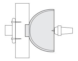
Cut a dovetail in the block to fit the spigot on the bowl.
