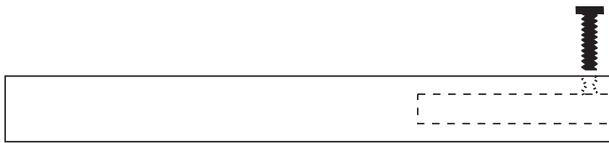
Drill and tap a hole to take a small bolt to hold the chatter blade in place. A 4mm bolt started 6mm back from the end is recommended. Cut the bolt to minimise any protrusion when it is tight.
