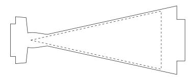
Turn the general shape between centres and make a spigot on both ends for use later in a scroll chuck. At the larger end allow some space in the design as the lower part of the box will need to slip down by the thickness of your parting cut and the overlap of the top if you wish to retain your designed proportions.
