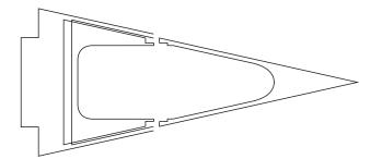
Remove the lid. Hollow and finish the inside. Check the fit of the lid.
