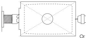
Start with a block of heavy wood 130mm long and 80mm thick both ways. The grain should lie along the long axis. Drill a 25mm hole through the centre. Mount this block between centres. Round it off and cut a spigot on one end.
