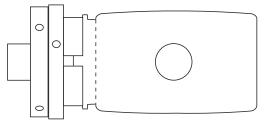
Mount in a chuck. Turn to a finished diameter of 70mm and create a little shape to the head. Round off the corners. Finish the outer face to be 55mm from the centre. Mark the line of the inner face. You may now part off and hand finish the other end or proceed to the next step.
