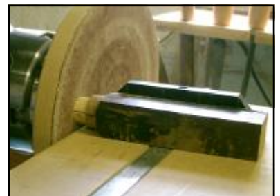
Photo 5- Using datum lines on sanding jig
