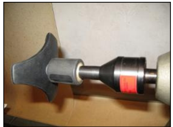
Adapted live centre mounted on tailstock ready for use
