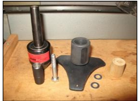
Left to right: Teknatool Nova Live Centre parts used in Johns adaptation, rubber walking stick tip, fabricated hardwood adaptor and washers
