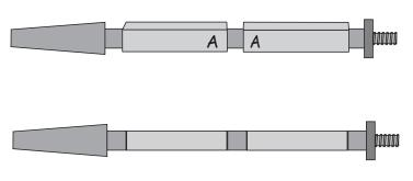
Use the three bushings as shown. Keep the Grain Markers together as this is the way the grain will be on the finished pen. Tighten the knurled knob to secure the pen Parts and bushings on the Mandrel.
