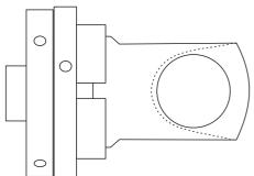
Now turn it down to the required diameter and cut the face to the desired shape.
