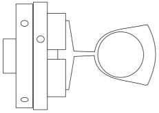
Cut around the ring keeping even thickness but then thicker at the bottom where it is weaker end grain wood. Part/saw it off.
