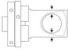
Mount the wood in a chuck and turn it to round. Check the wall thickness on both sides of the ring. If they are not equal then shift the wood in the chuck.
