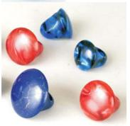
A single slash through a coloured surface is achieved with one offset of the wood in the chuck.
